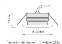
Light source Code FAG-24-11-WW-W O Warm white: 11W LED brand LG | 3000 K O Natural white: 11W LED brand LG | 4000 K FAG-24-11-NW-W FAG-24-11-CW-W Cool white: 11W LED brand LG | 6000 K RGB: 11W LED brand CREE FAG-24-11-RGB-W RGBW: FAG-24-16-RGBW-W 16W LED brand CREE
